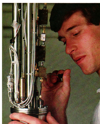
Final adjustments are made to the superfluid helium acoustic microscope cryostat before cooling.
